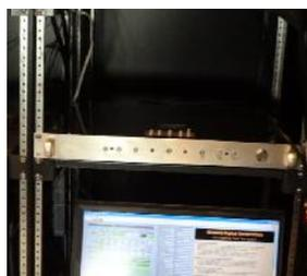
Figura 14 – Receptor digital profissional HD Radio
